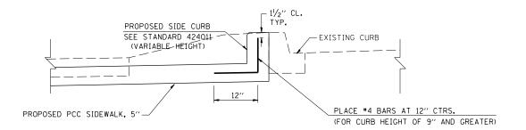
SIDEWALK CURB DETAIL TO BE USED ON IL 37 AT DIRTBUSTER CARWASH AND CVS PHARMACY. (SEE IL 37 CROSS SECTIONS)
