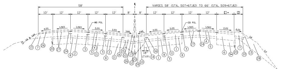
STA. 506+92.82 EB TO STA. 521+38.92 EB STA. 504+07.00 WB TO STA. 510+34.00 WB \* [] SHOULDER PAVEMENT & SUB-BASE WIDTH VARY [2] 10' (STA. 509+17.82) TO 12' (STA. 509+67.82) VARIES 0' (STA. 507+67.82) TO 6' (STA. 509+17.82)
