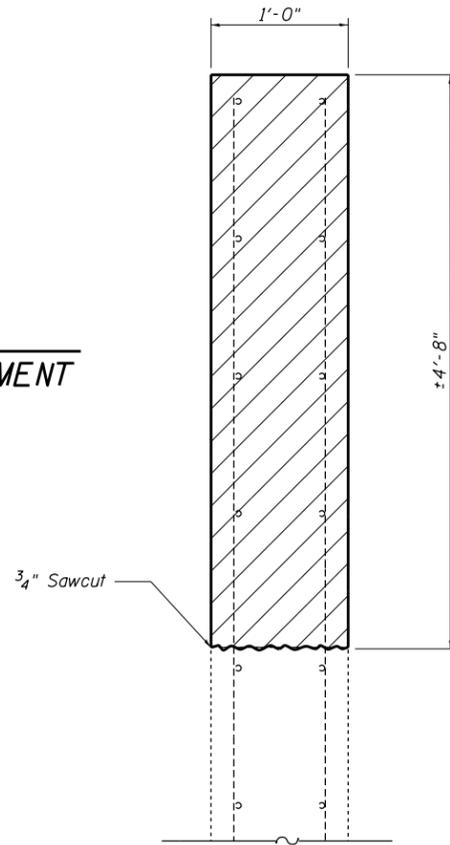
Hatching indicates Concrete Removal.
