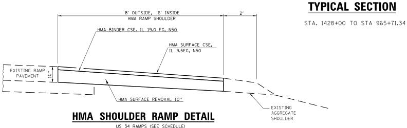
НМА НМА SURFACE FOR BINDER FOR SHOULDERS SHOULDERS BOTTOM LIFTS TOP LIFTS PG GRADE PG64-22 PG64-22 DESIGN AIR 4.0% € 4.0% € VOIDS N50 N50 IL 9.5 FG MIXTURE IL 19.0 FG COMPOSITION FRICTION AGGREGRATE MIXTURE C DENSITY CONTROL CORES/ CORES
