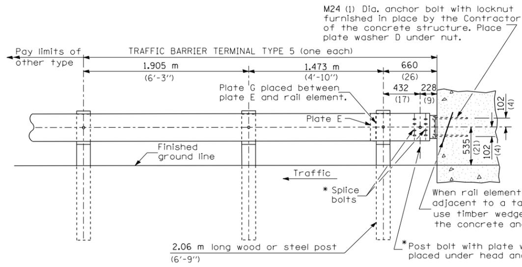
**TYPE 5 - CONCRETE BRIDGE PARAPET**
