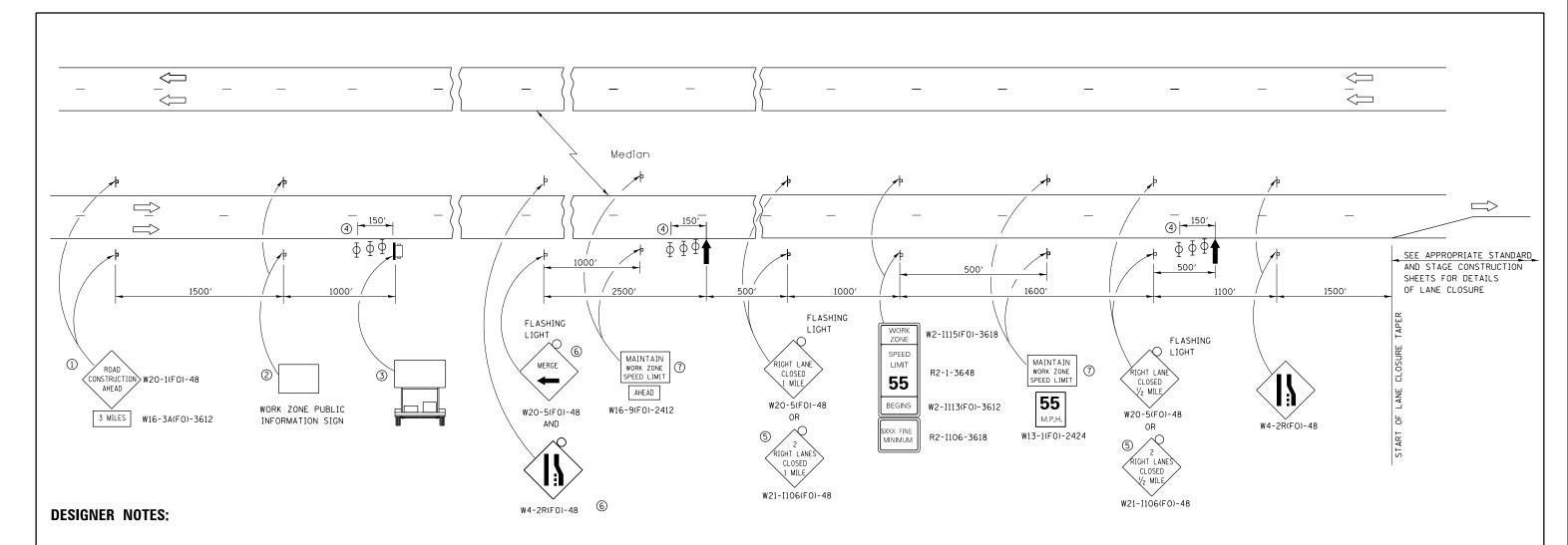
DETAIL 701–10 IS TO BE USED ON ALL INTERSTATE PROJECTS. THE BUREAU OF CONSTRUCTION SHALL DETERMINE EITHER OPTION 1 OR 2.
