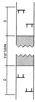
Type III Barricades and R11-2-4830 signs are to be shown at Road Closed to Thru Traffic detail on Highway Standard 701901. If the distance "D" exceeds 2000', an additional set of barricades and R11-2-4830 shall be placed at each end of the work area.
