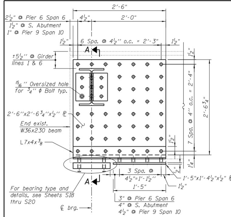
**DIAPHRAGM AND GIRDER REPAIR DETAIL**
