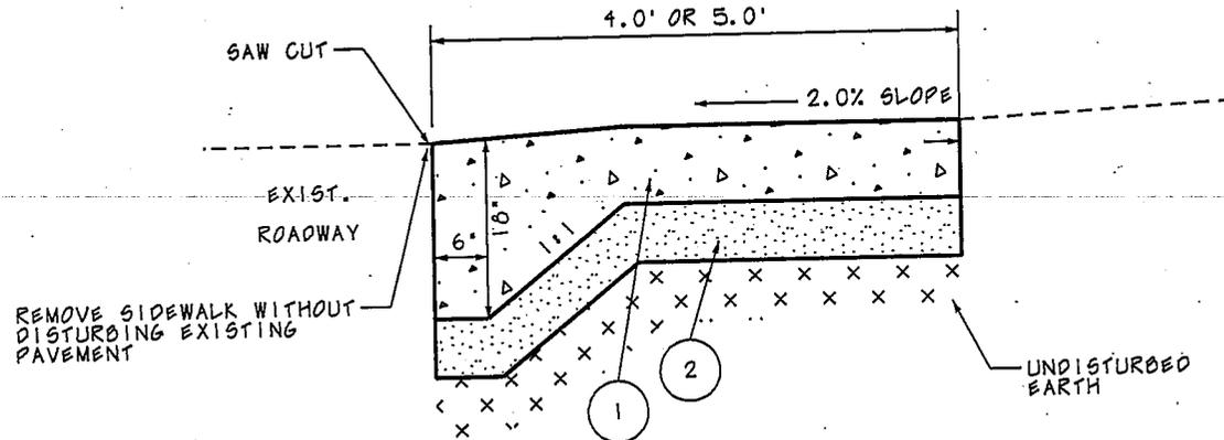
1. P.C.C. CLASS S1 - 6 INCH THICK. PAID FOR AS P.C.C. SIDEWALK, 5 INCH (SPECIAL).
