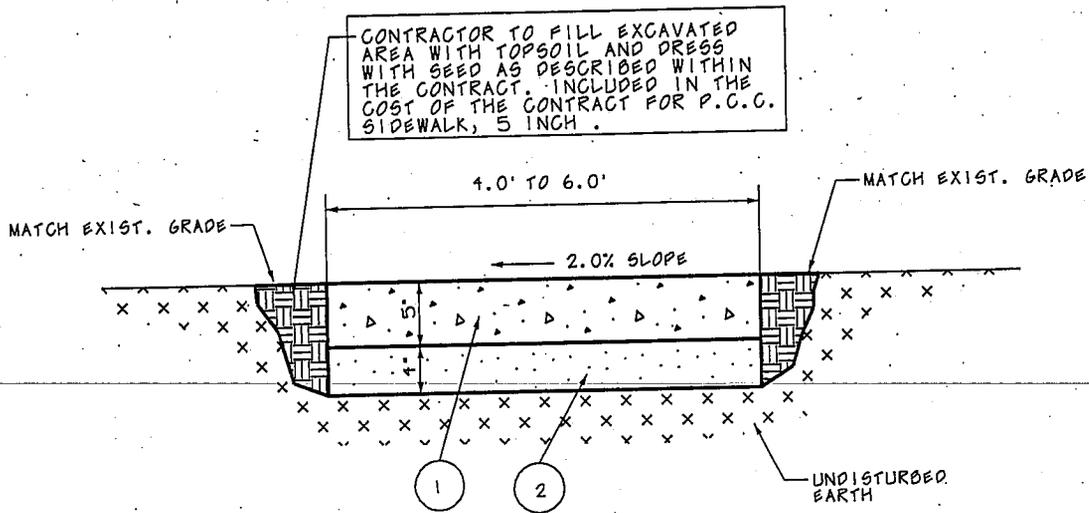
1. P.C.C. CLASS S1 - 6 INCH THICK. PAID FOR AS P.C.C. SIDEWALK, 5 INCH.
