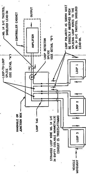
DETECTOR LOOP WIRING SCHEMATIC
