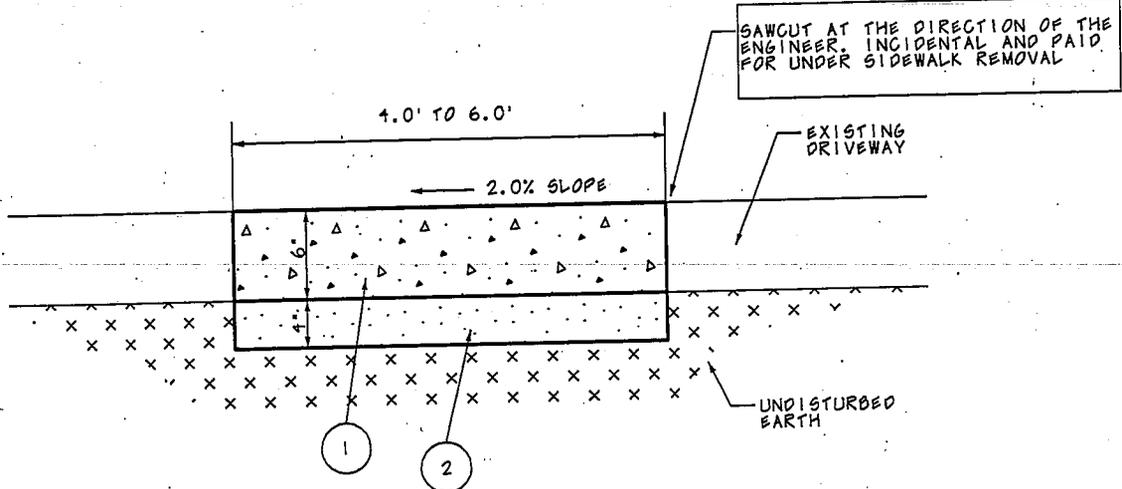
1. P.C.C. CLASS S1 - 6 INCH THICK. PAID FOR AS P.C.C. SIDEWALK, 5 INCH.
