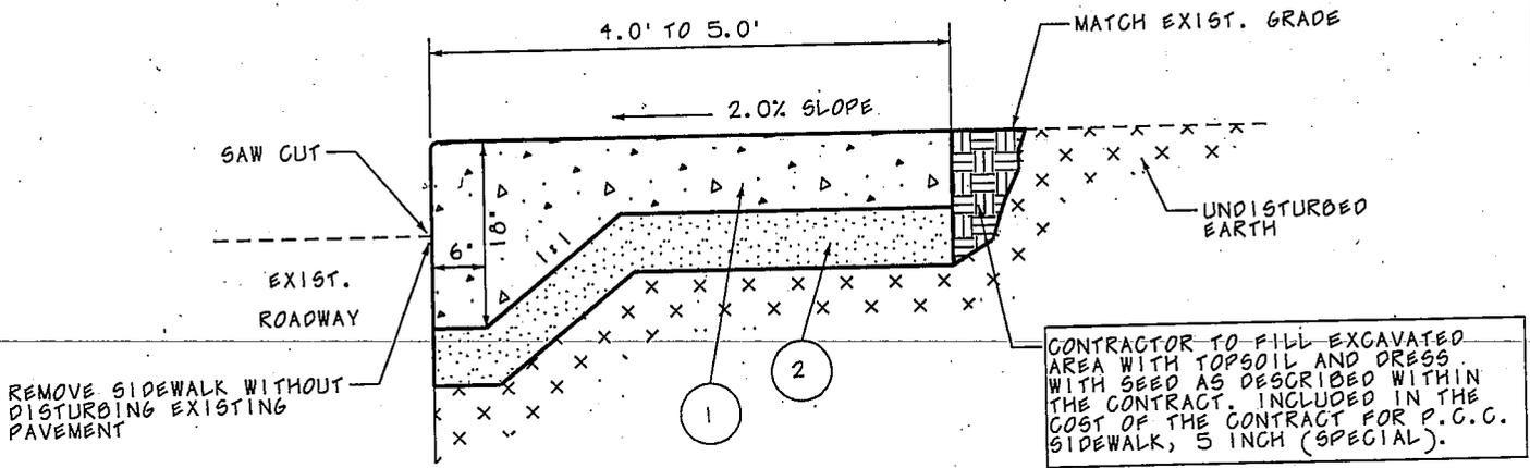
1. P.C.C. CLASS S1 - 6 INCH THICK. PAID FOR AS P.C.C. SIDEWALK, 5 INCH (SPECIAL).
