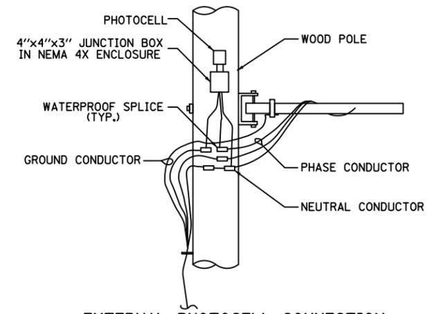
**EXTERNAL PHOTOCELL CONNECTION AND MOUNTING DETAIL (FOR HIGH MAST LUMINAIRE ONLY)**
