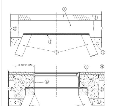
EXISTING BROKEN FRAMES AND LIDS SHALL BE REMOVED AND DISPOSED OF BY THE CONTRACTOR AND SHALL BE REPLACED AS DIRECTED BY THE ENGINEER. REPLACEMENT FRAMES AND LIDS WILL BE PAID FOR IN ACCORDANCE WITH ARTICLE 109.04 OF THE STANDARD SPECIFICATIONS UNLESS A SEPARATE PAY ITEM HAS BEEN PROVIDED.
