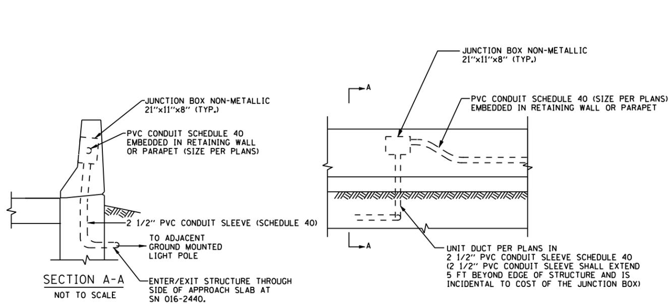
**UNDERGROUND TO EMBEDDED CONDUIT TRANSITION**
