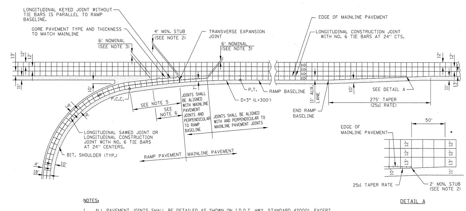
1. ALL PAVEMENT JOINTS SHALL BE DETAILED AS SHOWN ON I.D.O.T. HWY. STANDARD 420001, EXCEPT EXPANSION JOINT SEALS SHALL BE AS DESCRIBED IN THE SPECIAL PROVISION, BONDED PREFORMED JOINT SEALER.
