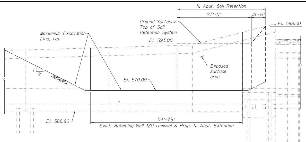
**TEMPORARY SOIL RETENTION SYSTEM 1 ELEVATION**
