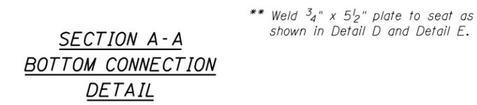
\*\* Weld 3/4" x 5 1/2" plate to seat as shown in Detail D and Detail E.
