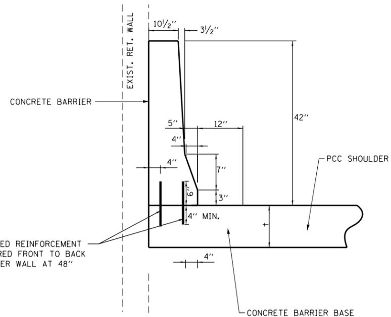
**CONCRETE BARRIER BASE DETAIL
