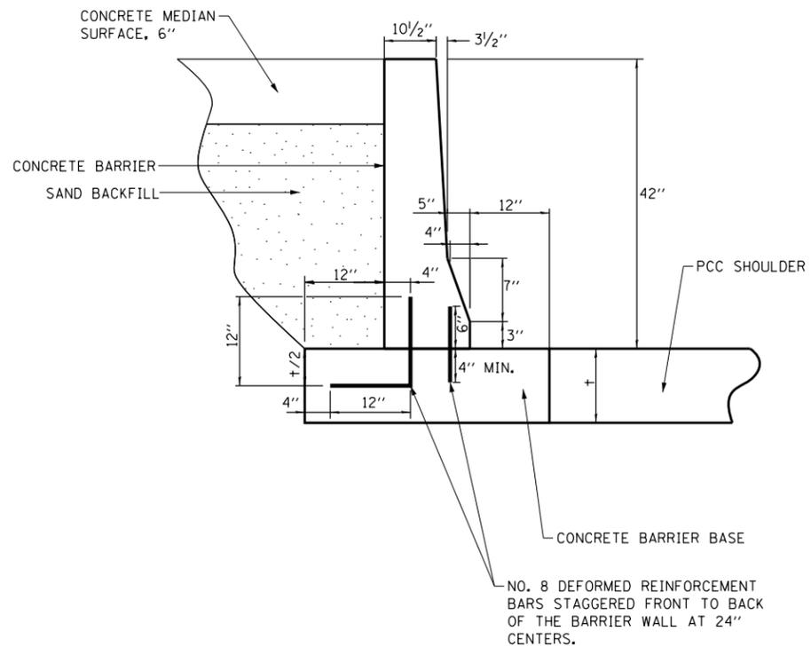
**CONCRETE BARRIER BASE DETAIL
