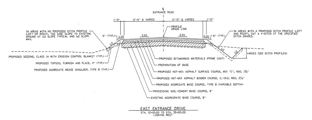
\*NOTE: AGGREGATE BASE COURSE, TYPE B WILL BE PLACED AT A THICKNESS OF B" FROM STA. 10+10.00 TO STA. 11+00.00.
