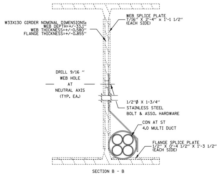
W33X130 GIRDER DIMENSIONS REQUIRE FIELD VERIFICATION PRIOR TO WEB DRILLING, CLAMP FABRICATION AND SELECTING FASTENING HARDWARE
