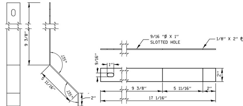
CLAMP MATERIAL MUST BE COMPATIBLE W/THE GIRDER MATERIAL
