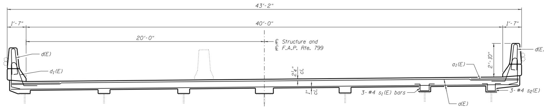
SECTION B-B BENT 6-EAST SPAN
