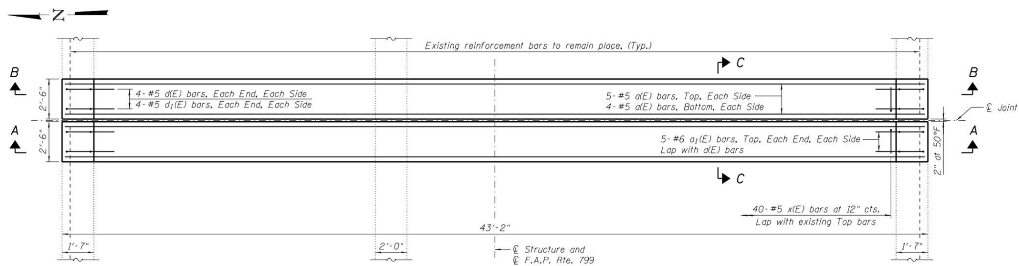
**PLAN AT BENT W, 2, 3-WEST SPAN, 17, 18, 22, 23, 27, AND 28**
