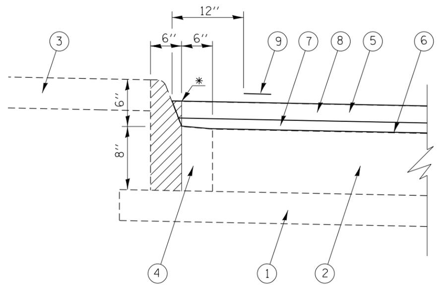
**PROPOSED CONCRETE CURB REPAIR DETAIL
