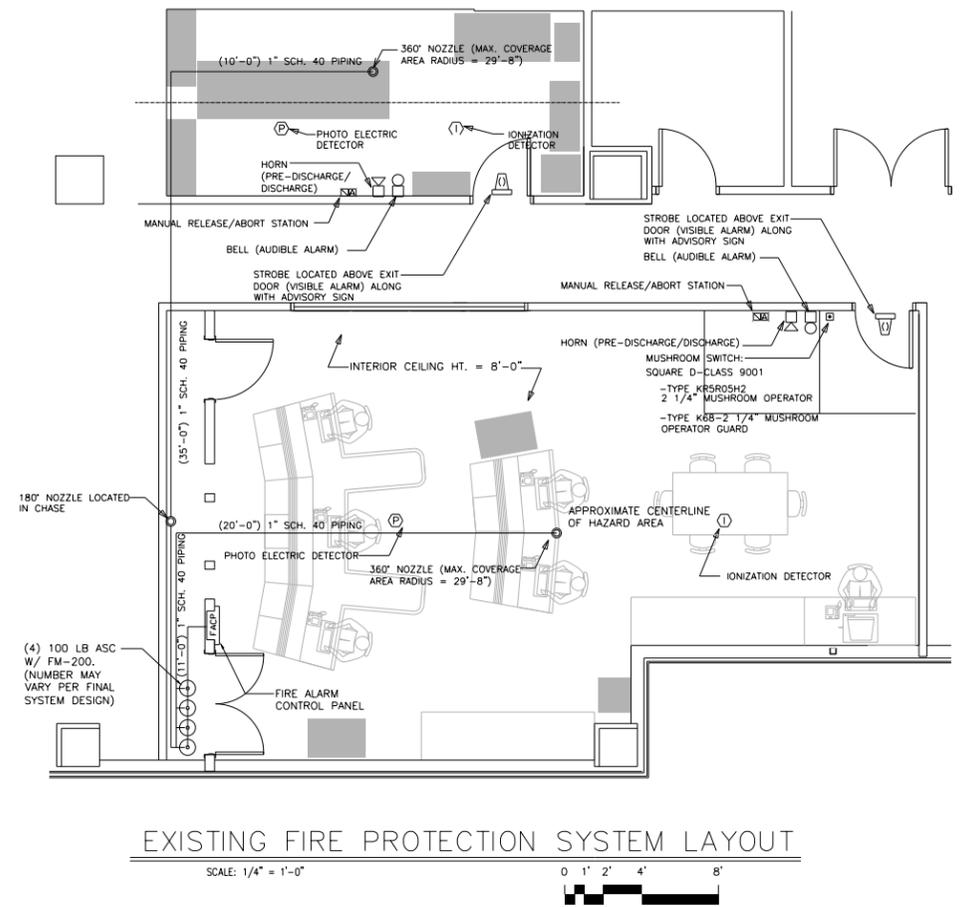
(4) 100 LB CLEAN AGENT STORAGE CONTAINERS (ASC), W/ PRESURE GAUGE AND 1" VALVE ASSEMBLY. EACH CONTAINER FILLED WITH FM-200. CONTAINERS TO BE FASTENED TO WALL OR OTHER SECURE SURFACE BY MEANS OF U-SHAPED MOUNTING BRACKETS. (APPROX. SIZE OF ONE 100LB TANK IS 10.75" DIA. X 38.75" HT.)
