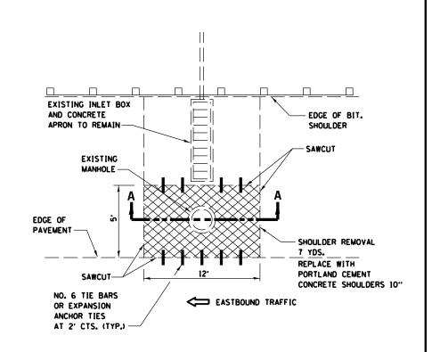
THE WORK SHOWN HERE SHALL BE INCLUDED IN THE CONTRACT UNIT PRICE PER SO YD FOR SHOULDER REMOVAL AND PORTLAND CEMENT CONCRETE SHOULDERS 10".
