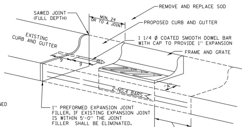
WHEN "A" IS GREATER THAN 2', 2-NO. 4 BARS SHALL BE PLACED AS SHOWN.
