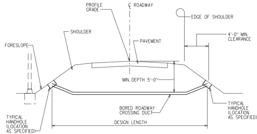
TYPICAL ROADWAY TRANSVERSE SECTION WITH HANDHOLE ON SLOPE
