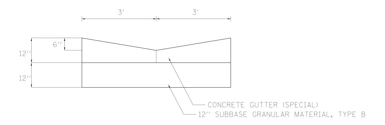
NOTES: THIS WORK SHALL BE DONE IN ACCORADNACE WITH THIS DETAIL AND STANDARD 606101
