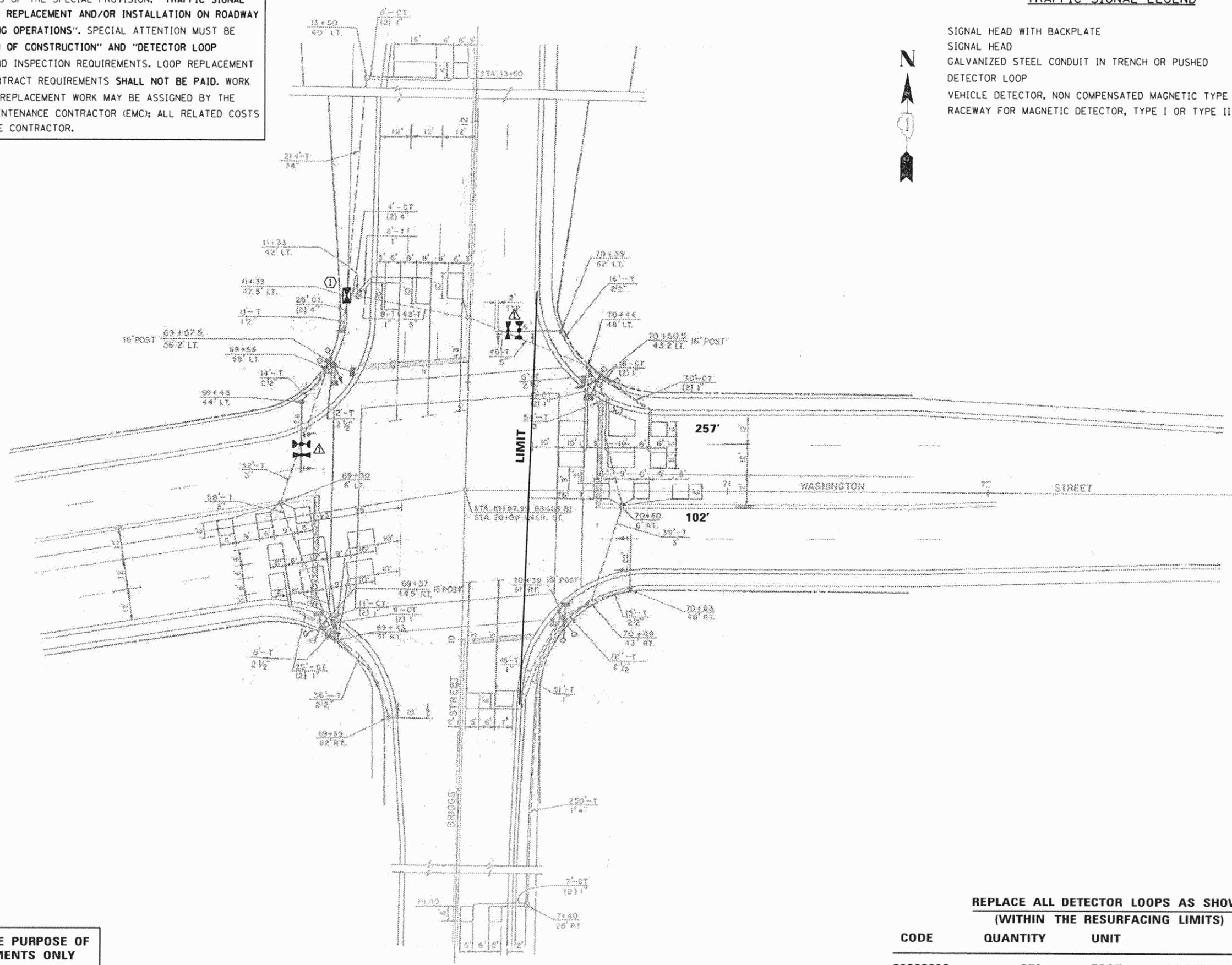
**THIS PLAN IS FOR THE SOLE PURPOSE OF DETECTOR LOOP REPLACEMENTS ONLY**
