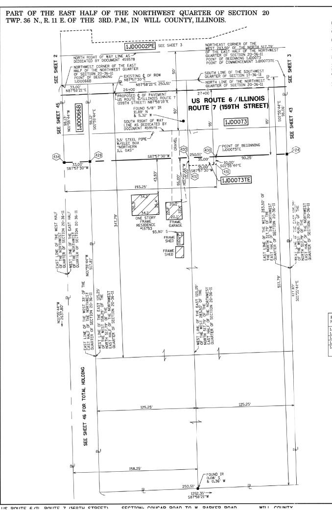
PROJECT COORDINATE VALUES AND BEARINGS ARE GROUND AND BASED ON ILLINOIS STATE PLANE, EAST ZONE, REFERENCE ELLIPSOID, WGS 1984 WITH A COMBINED SCALE FACTOR OF 0.9999544733.
