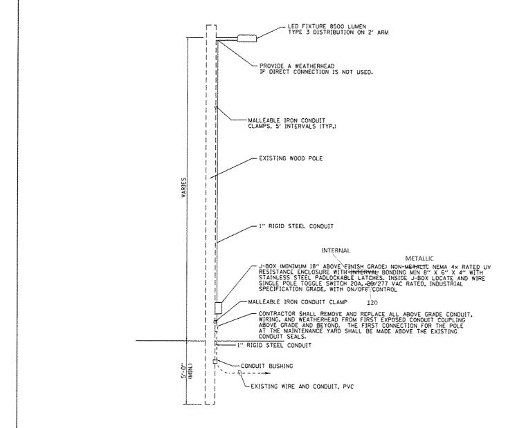
NOTE: CIRCUIT SHALL BE ADEQUATELY PROTECTED WITH A BREAKER AT THE SOURCE
