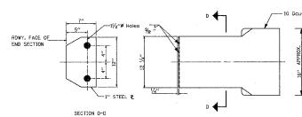
ALL OTHER STEEL SHAPES AND PLATES SHALL CONFORM TO THE REQUIREMENTS OF A.A.S.H.T.O. DESIGNATION M-183 EXCEPT POSTS AND ANGLES SHALL CONFORM TO A.A.S.H.T.O. M-223, GRADE 50.
