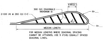
DIAGONAL LINE SPACING: 15 m (50') C-C (LESS THAN 50 km/h (30 MPH)) 25 m (75') C-C (50 km/h (30 MPH) TO 70 km/h (45 MPH)) 45 m (150') C-C (MORE THAN 70 km/h (45 MPH))
