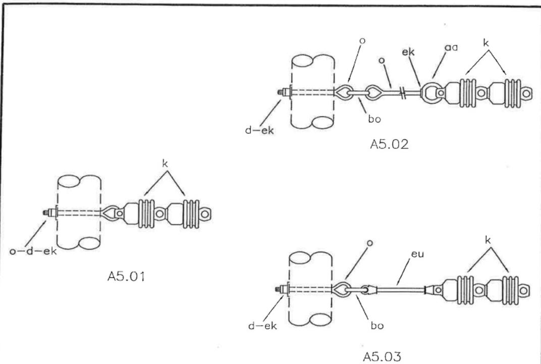
NOTE: When connecting to existing bolt end, use eye nut "aa" and locknut "ek" instead of eyebolt subassembly "o-d-ek".
