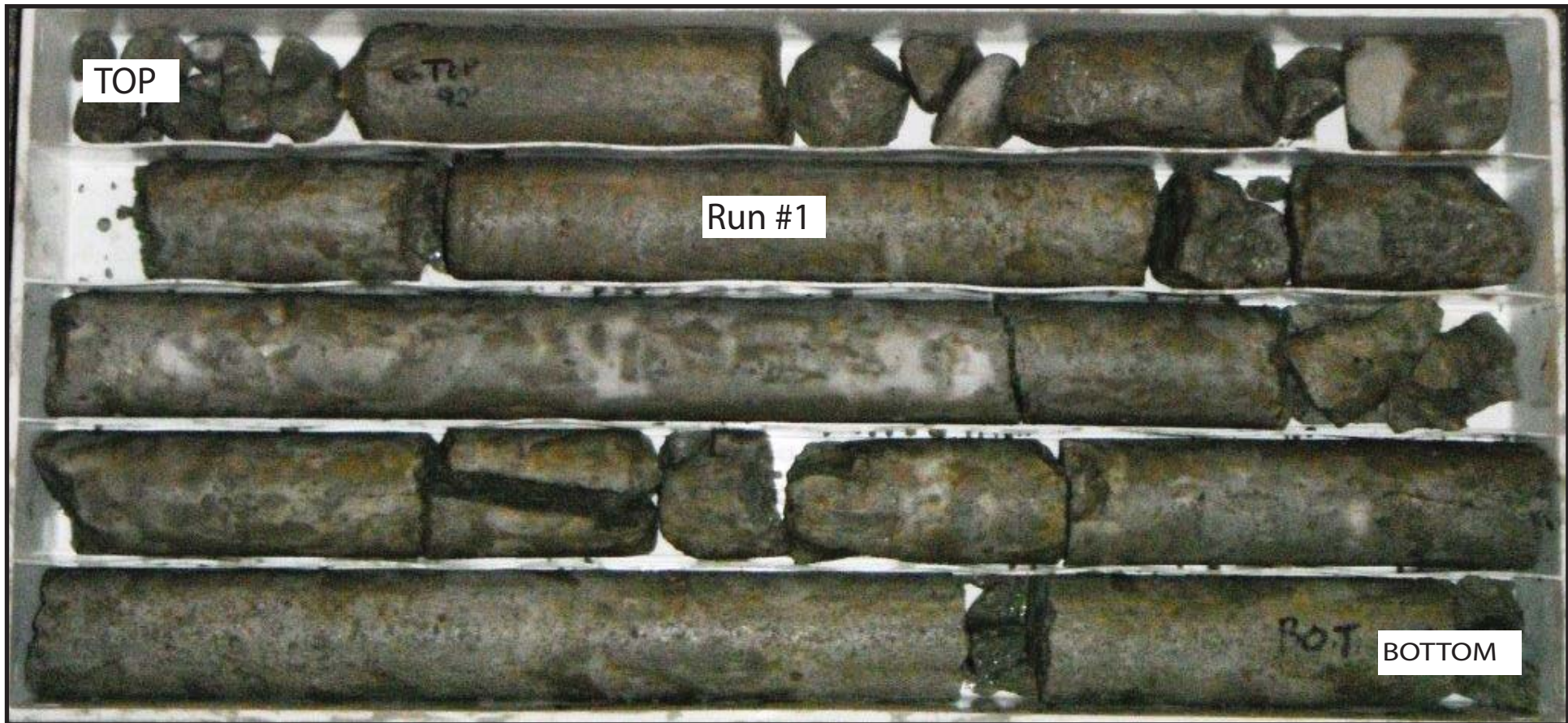
Boring 1702-B-02 Run #1, 92' to 102', RECOVERY = 99% , RQD = 57%
