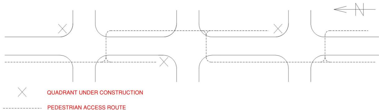
Only one quadrant per block is under construction. This allows access to every building on the main route and an uninterrupted pedestrian access route.
