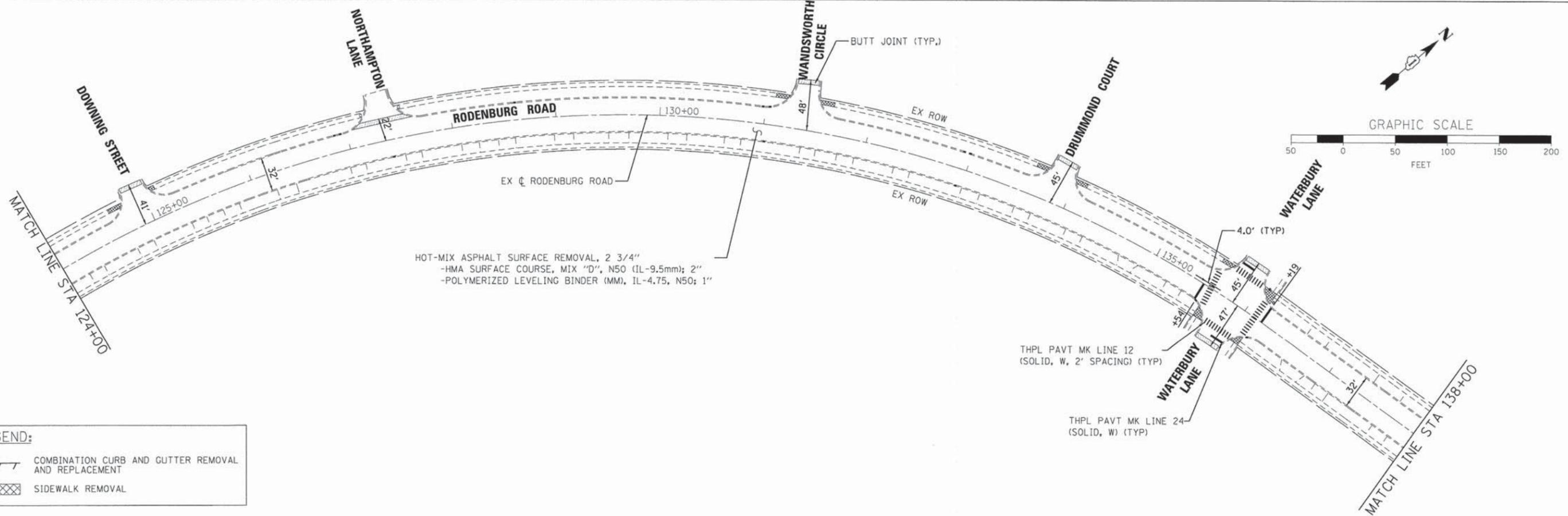
HOT-MIX ASPHALT SURFACE REMOVAL, 2 3/4"
