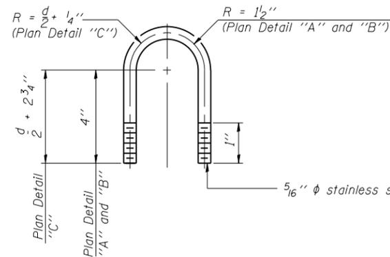
**DAMPING DEVICE MOUNTING TUBE U-BOLT DETAIL**
