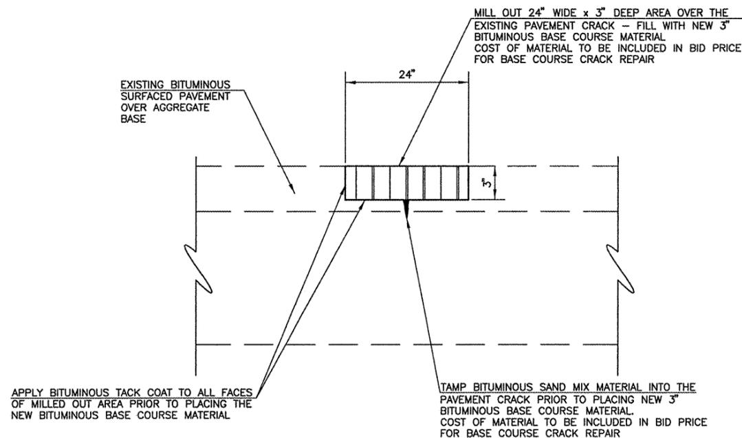
**BASE COURSE CRACK REPAIR DETAIL**
