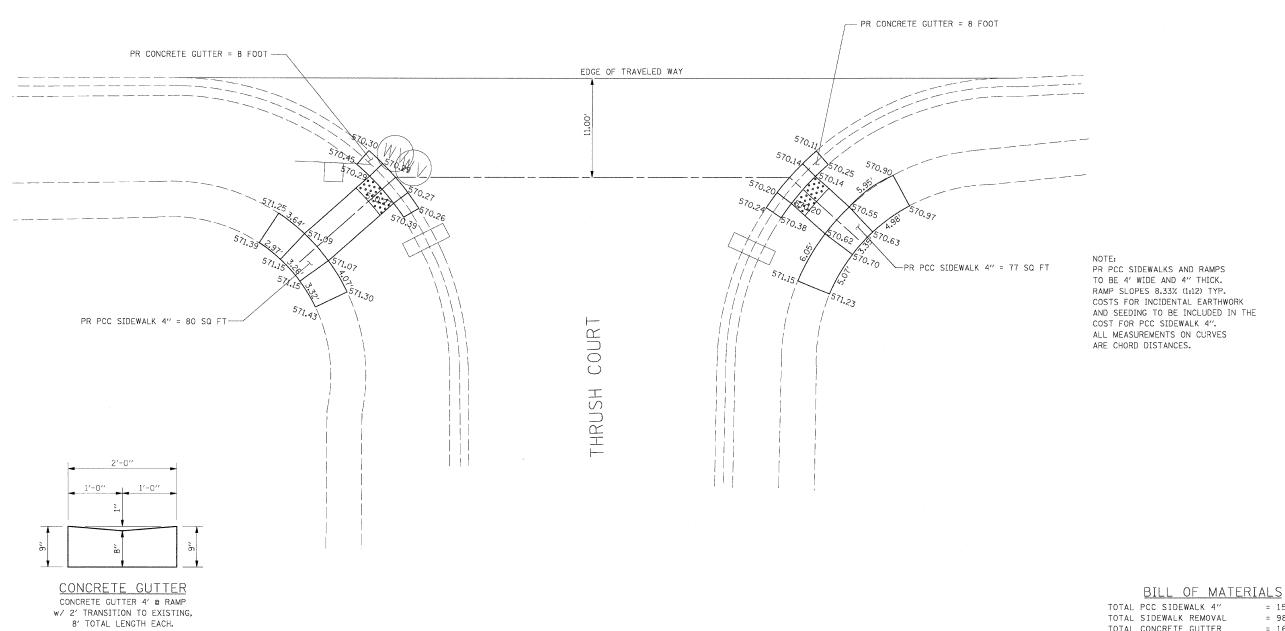
TOTAL PCC SIDEWALK 4" = 157 SQ FT = 98 SQ FT = 16 FT = 16 FT TOTAL SIDEWALK REMOVAL TOTAL CONCRETE GUTTER TOTAL GUTTER REMOVAL
