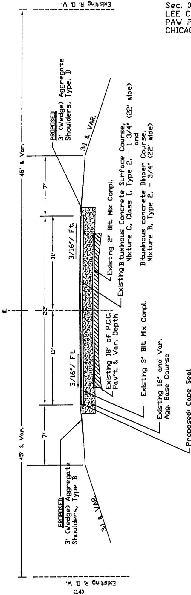
**CONSTRUCTION NOTE:** THE THICKNESS OF THE BITUMINOUS MIXTURE SHOWN ON THE PLANS IS THE NOMINAL THICKNESS. DEVIATIONS FROM THE NOMINAL THICKNESS WILL BE PERMITTED WHEN SUCH DEVIATIONS OCCUR DUE TO IRREGULARITIES IN THE EXISTING SURFACE ON WHICH THE BITUMINOUS MIXTURE IS PLACED.
