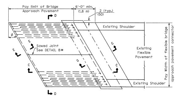
BRIDGE APPROACH PAVEMENT CONNECTOR (FLEXIBLE)
