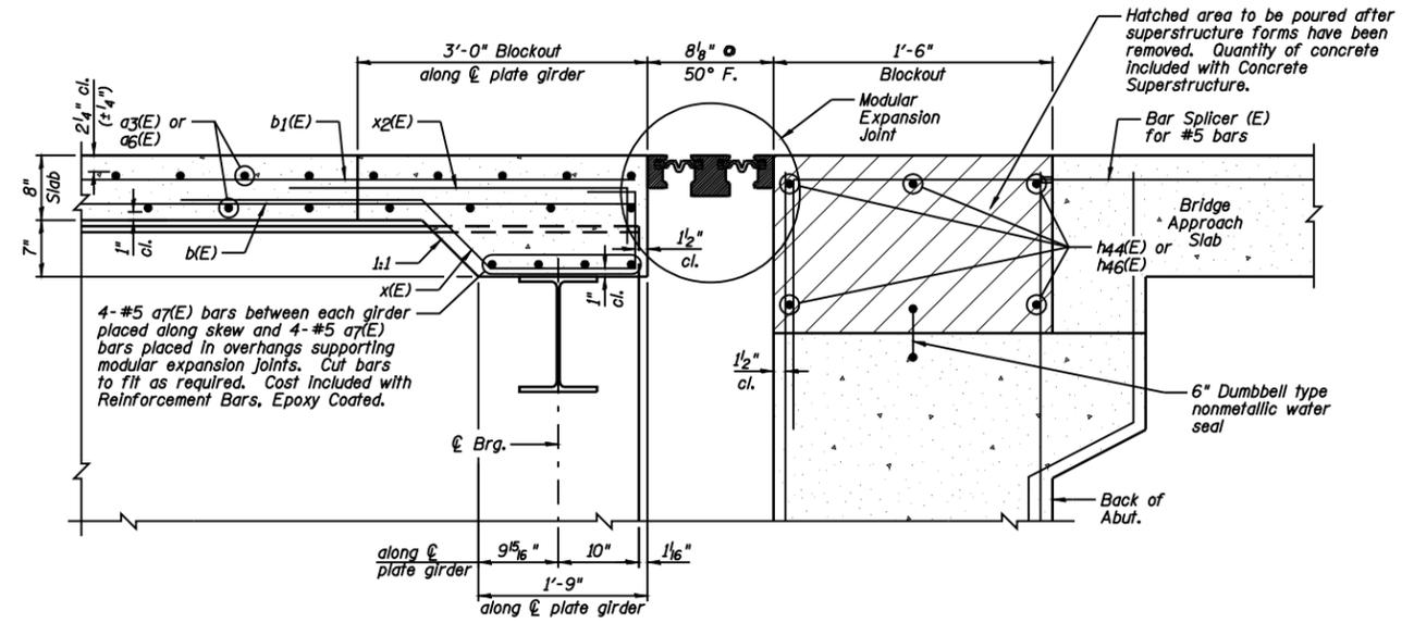
**SECTION THRU STRUCTURE AT NORTH ABUTMENT**
