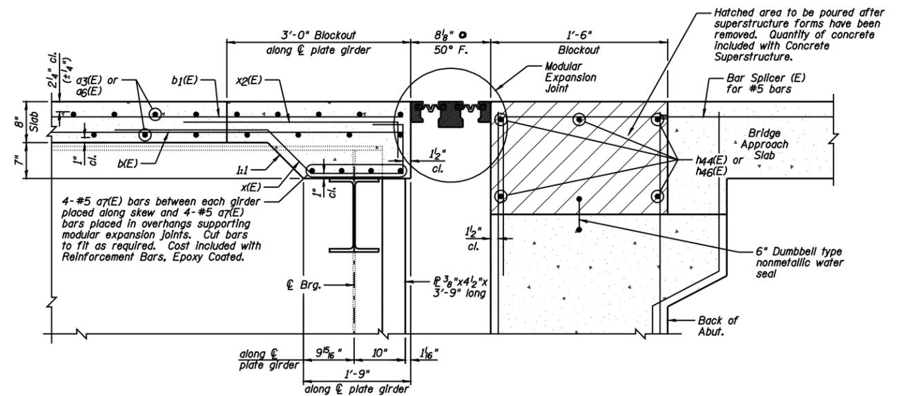
**SECTION THRU STRUCTURE AT NORTH ABUTMENT**
