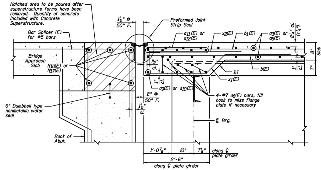
**SECTION THRU STRUCTURE AT SOUTH ABUTMENT**
