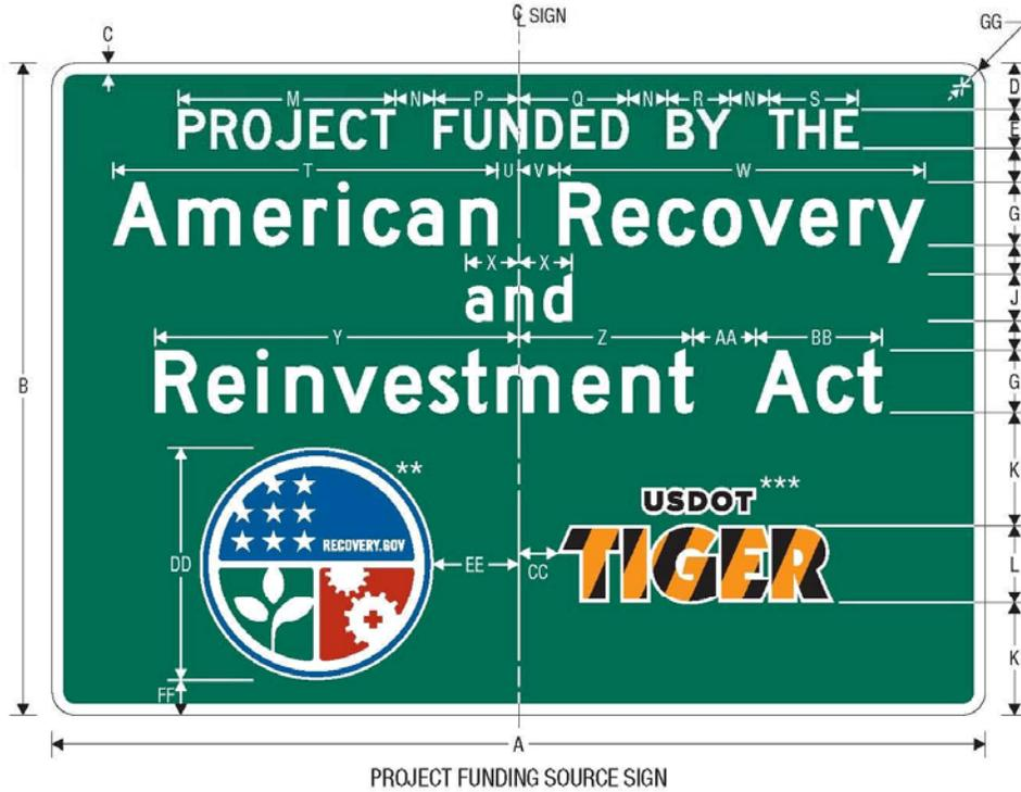
NOTE: SIGN SHALL NOT BE INSTALLED WITHOUT PROJECT FUNDING SOURCE PLAQUE
