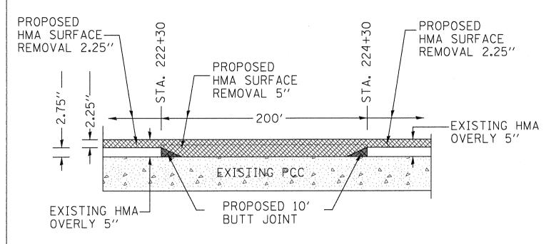
1 AT THIS LOCATION; EXISTING HMA OVERLAY WILL BE MILLED TO THE EXISTING PCC
