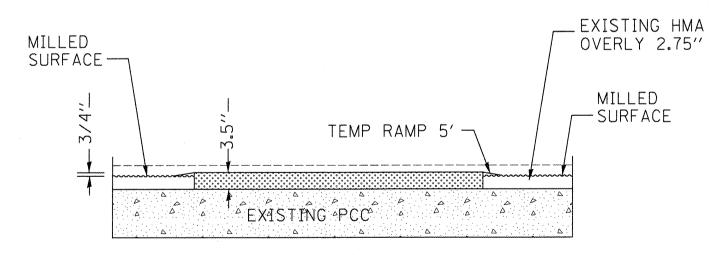
2 PROPOSED HMA BINDER COURSE WILL BE PLACED APPROXIMATELY 3.5" DEEP. THIS LIFT OF BINDER COURSE SHALL BE 3/4" ABOVE THE ADJACENT MILLED SURFACE
