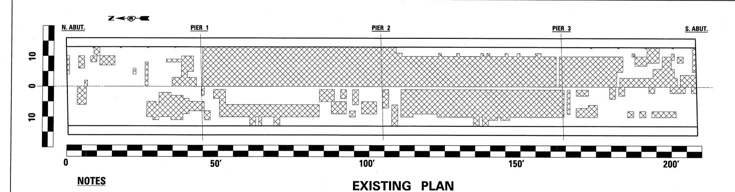
CROSS HATCHED AREA REPRESENTS ESTIMATED DECK SLAB REPAIR (PARTIAL DEPTH).
