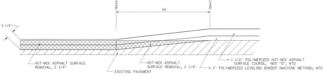
DESIGNED SECTION DRAWN REVISED STATE OF ILLINOIS 553 120M PROPOSED TYPICAL SECTION PLOT SCALE = 20.0000 '/ IN. CHECKED REVISED **DEPARTMENT OF TRANSPORTATION** CONTRACT NO. 64E55 PLOT DATE = Tue Jan 13 15:38:59 2009 REVISED SHEET NO. OF SHEETS STA. TO STA.
