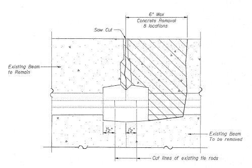
BEAM REMOVAL DETAIL AT TRANSVERSE TIES
