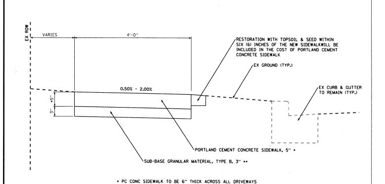
.. INCLUDED IN THE COST OF PORTLAND CEMENT CONCRETE SIDEWALK, 5 INCHES PORTLAND CEMENT CONCRETE SIDEWALK
