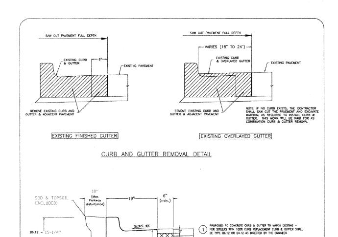
COMBINATION CONCRETE CURB AND GUTTER DETAIL
