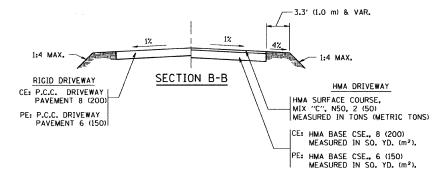
RURAL FIELD ENTRANCE (FE) HMA SURFACE COURSE. MIX "C", N50, 2 (50) MEASURED IN TONS (METRIC TONS) AGGREGATE BASE CSE., TYPE B, 8 (200) MEASURED IN SO. YD.  $(m^2)$ .
