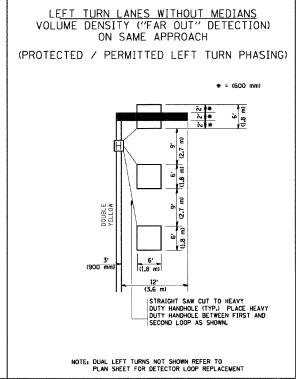
CROSS STREET-VOLUME DENSITY ("FAR OUT" DETECTION) ARTERIAL CALLING LOOP IN RIGHT TURN LANE. CROSS STREET [TYP.-12' (3.6m) LANES] 12' 12' 12' 12' 12' 3.6m) (3.6m) [TYP.-ALL LEGS-VOLUME ("FAR OUT" DETECTION)] DUCT IS RUN BETWEEN EDGE OF PAVEMENT STRAIGHT SAW CUTS TO HEAVY-DUTY HANDHOLE-DRIVEWAY AND HANDHOLE. OFF SET LOOPS BY IN PAVEMENT THAT TERMINATE IN HANDHOLES STRAIGHT SAW CUTS. OUTSIDE PAVEMENT)
